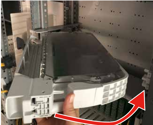
2 Refermer le battant Close the swiveling chassis
