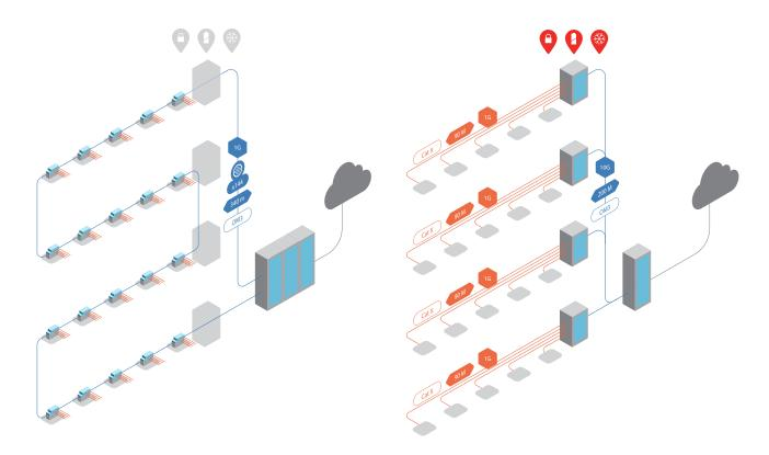
Passive fibre cabling and active switches are combined to provide Gigabit Ethernet services from the central core switch to an FTTO switch and from there to end user devices.
