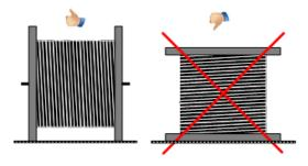
Laying the reel on its side may cause damage to the reel flange and/or cause the OF cable layers to shift - This may cause cable to snag during de-reeling.
