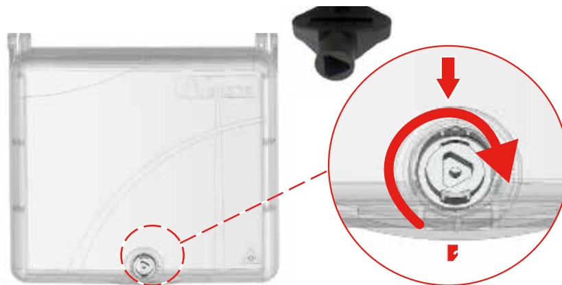
Fig. Fermeture du boîtier OutDrop 2+ Epissurage Closing the OutDrop 2+ Epissurage device
